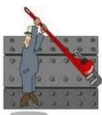
Adjustable wrenches are not made for hard service, so set the adjusting knurl so the wrench fits the nut snugly. Grip the nut or bolt so that the pulling force is applied to the stationary jaw section. Pulling the wrench is recommended over pushing it.
